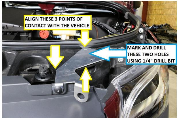
5) With holes drilled, install the included ¼-20 x 1" long button head bolts with a washer under the bolt head. Install a flange nut on the underside of the core support. Snug the front Torx bolt first, then snug the button head allen bolts using a 5/32" allen. See image below of installed front bracket.
