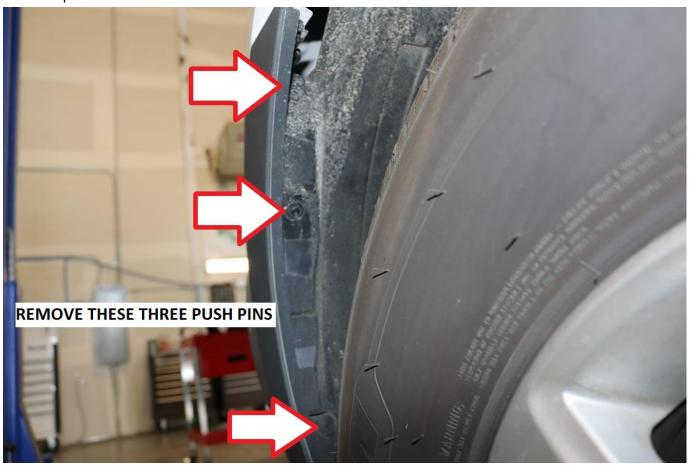
11) Look up from the iniside of the fender where the plastic bumper cover meets the metal fender and locate the last remaining push pin securing the bumper cover to the vehicle.
