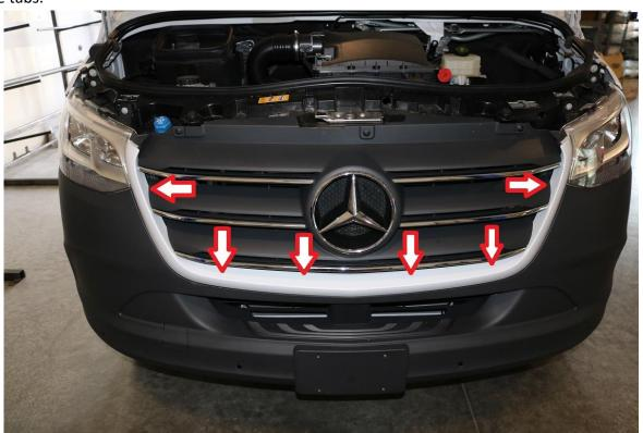
3) Once these tabs are located, push down on them and gently pull the bottom of the grill away from the van and it should come free from the vehicle. We have found a long flat nose screwdriver to work well as a tool to push down on the tabs.
