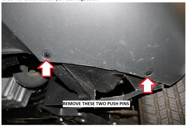
9) Use an automotive trim removal tool to pry up under the head of the push pin prior to prying under the body of the fastener to fully remove it.
