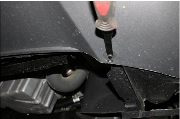
10) Next, on the inside of the fender well, remove the three push pin fasteners near the outer lip of the bumper.
