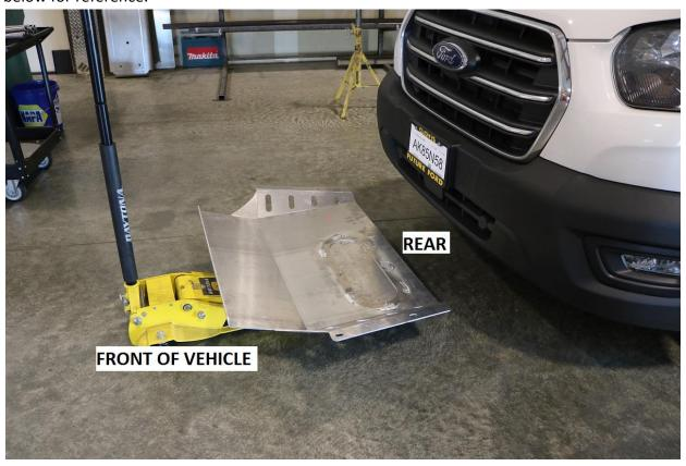
6) Fit the skid plate to the bumper support bars as shown using the M12 hardware included in the kit.
