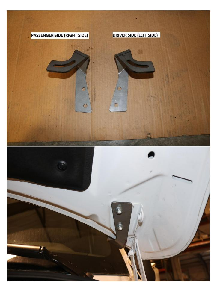
4) Once the bracket and nuts have been installed, torque the nuts using a 13mm socket to 13 ft-lbs (17.6 N.m)
