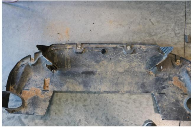
10) With the top scoop removed, trim the lower air deflector as shown below. Measure over 1" from the rear mounting bolt access holes and mark out a rectangle as shown.
