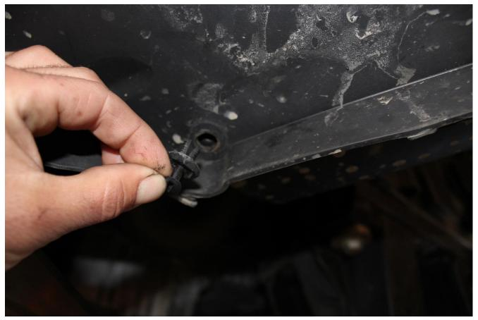
8) Next, on the inside of the fender well, remove the three push pin fasteners near the outer lip of the bumper cover.
