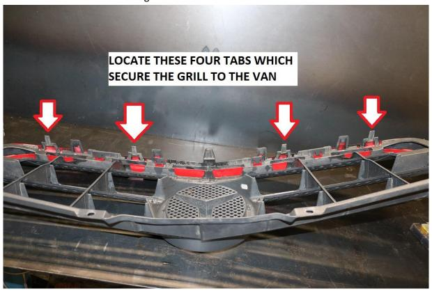
4) Once these tabs are located, push down on them and gently pull the bottom of the grill away from the van and it should easily come free from the vehicle. We have found a long flat nose screwdriver to work well as a tool to push down on the tabs.
