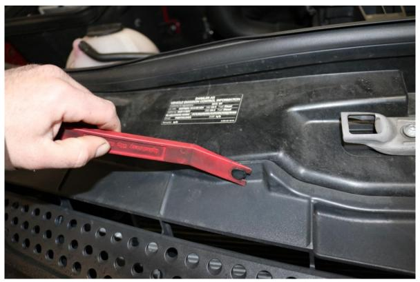
3) With the upper part of the grill separated, gently pull the top of the grill back and locate the four tabs which secure the bottom of the grill to the van.
