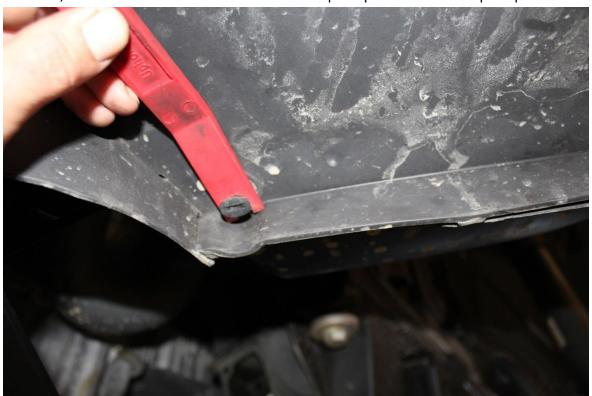
7) Using the same automotive trim removal tool, pry up under the head of the push pin body to fully removal the fastener. Remove these from both sides of the vehicle.
