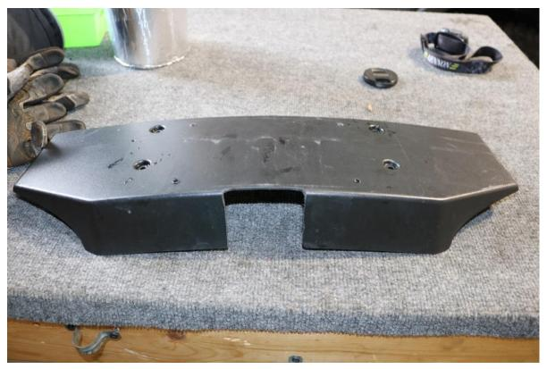
54) Fit and mark the outer cut profile of the winch fairlead on the license plate mounting panel.
