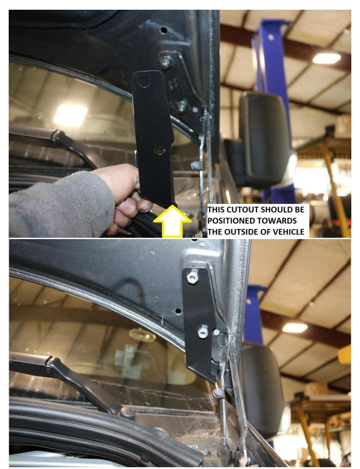
4) Once the bracket and nuts have been installed, torque the nuts using a 13mm socket to 10 ft-lbs (13.5 N.m)
