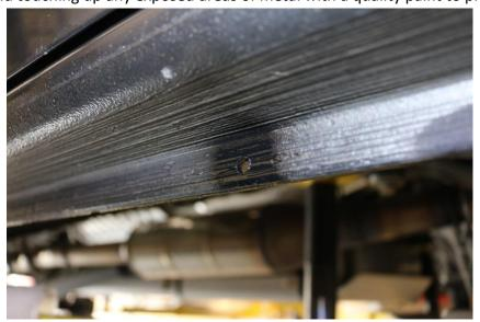
8) Assemble the top and bottom plates off the vehicle by installing all of the outer bolts only. Just install the outer bolts and start the nuts. Do not tighten them at this time. Use a washer under the bolt head. Use a 5/32" allen tool and the included 402206-01 install tool / wrench to aide in nut installation.
