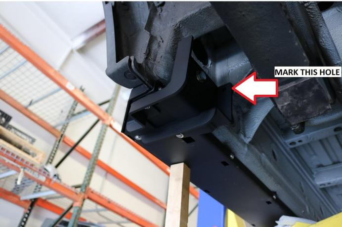
26) Snug all the attachment bolts and mark the front gusset hole on the body as referenced above. 27) Remove the rear chassis tie in from the vehicle and drill this hole with a 7/16" (11mm) drill bit.
