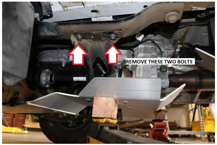
15) Install the 4022-03 Front Chassis Tie-in on the vehicle. These tie-in brackets are left and right specific and will only go on one way. Note image below for reference, showing the orientation of the bracket for the left side (driver side) of the vehicle.
