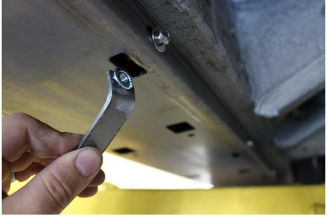
12) Once all inner and outer bolts have been installed with their respective flange nuts on the inside. Tighten the hardware. Torque all bolts to 80 in-lbs (9 N.m).
