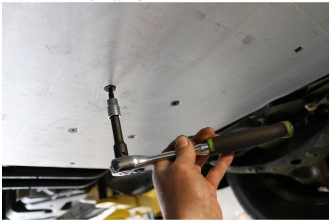
9) Install the 401001-05 front spacers. This is the shorter spacer. Install by placing the spacer in the access hole in the front cross member and sliding it over to line up with the mounting hole in the skid plate and cross member.
