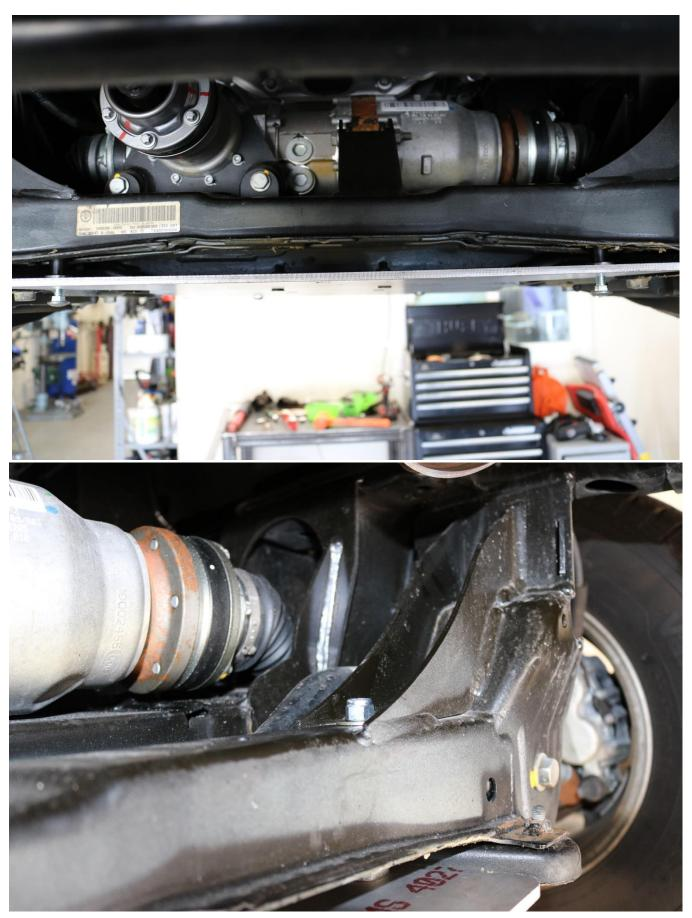
13) Snug all hardware at this time. Snug the flat head socket cap screws first, and then snug all the 3/8" nylock nuts. Use a 9/16" socket or wrench to tighten the carriage bolt hardware.
