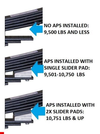
22) Note: **ALWAYS** install the slider pad with the countersunk holes on top as shown below.
