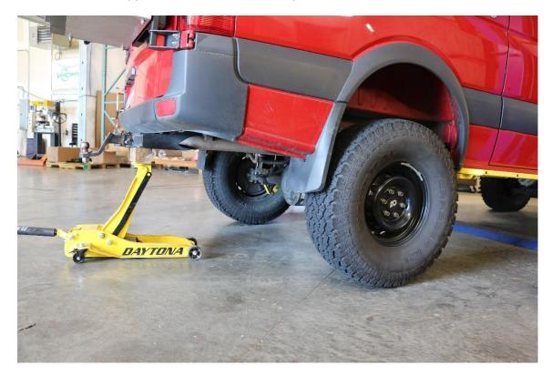
2) Note the shocks are left and right specific, refer to the part number etched on the shock body to ensure they are installed on the correct side.
