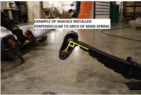
15) Install the leaf springs into the vehicle. We have found it easiest to install the springs upside down and then rotating them up into position once under the vehicle.
