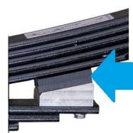
**APS INSTALLED WITH 2X SLIDER PAD:** 8,701 LBS & UP
