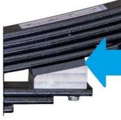
**APS INSTALLED WITH SINGLE SLIDER PAD:** 7,500 - 8,700 LBS
