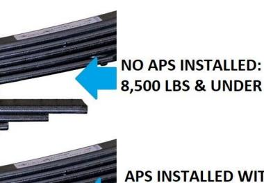
APS INSTALLED WITH SINGLE SLIDER PAD: 8,501 - 10,000 LBS
