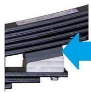
APS INSTALLED WITH 2X SLIDER PADS: 10,001 LBS & UP
