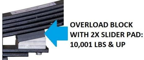
28) Note; **ALWAYS** install the slider pad with the countersunk holes on top as shown below.
