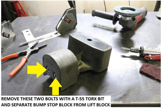
21) Identify LH & RH sides for the 3071 bump stop brackets included in the kit. Use the image below for identification.
