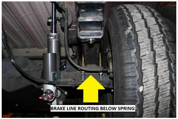
15) Once the springs are rotated into position. Install the forward spring bolt in the spring hanger, install the nut but do not fully tighten at this time.
