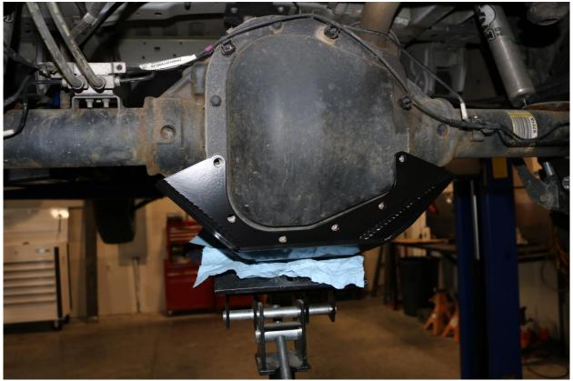
4) Install the included  $5/16-18 \times \frac{3}{4}$ " long bolts included in the kit with a washer under the bolt head. Start all 6 bolts and simply snug them down using a  $\frac{1}{4}$ " socket / wrench, do not fully tighten at this time, make sure the differential guard can still move.
