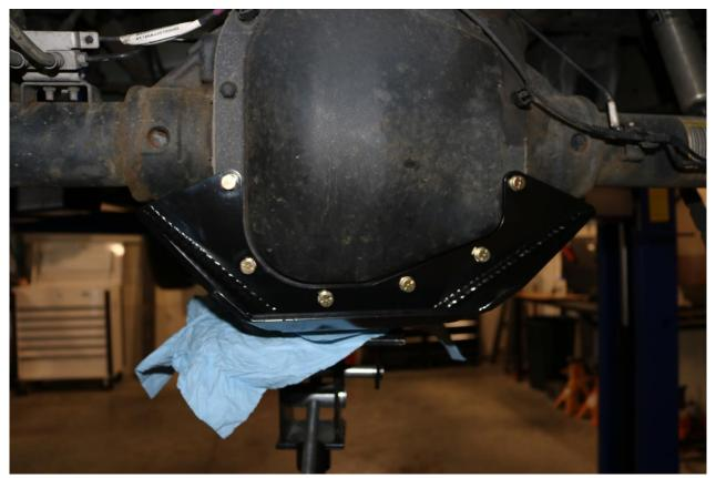
5) Use the floor jack to seat the front part of the differential guard against the bottom of the differential. Install the top pinion plate as shown.
