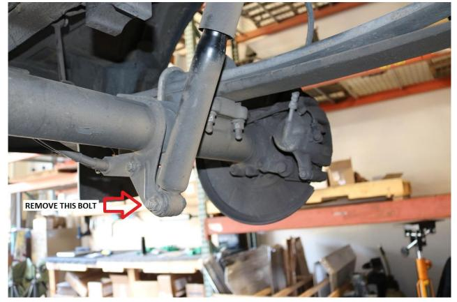
8) Remove the U-bolt nuts. Use a 19mm socket / wrench for removal. Remove the U-bolts. See image below.
