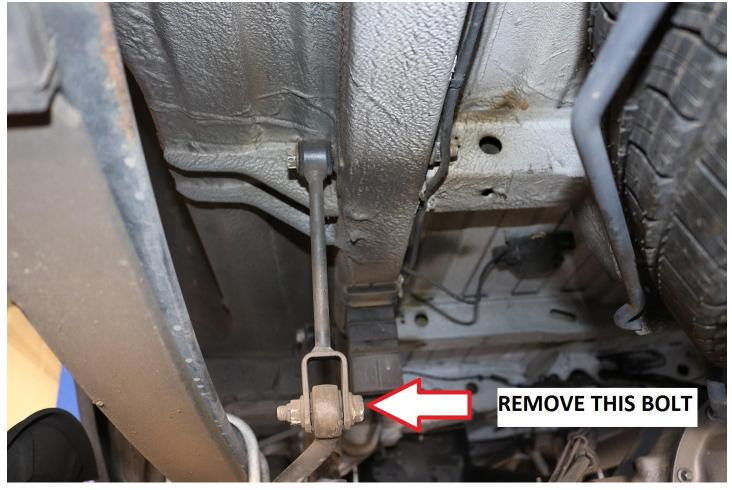
5) If equipped, disconnect the brake portioning / wind assist sensor lever. Retain the nut for future use. Use a 16mm socket / wrench for removal.
