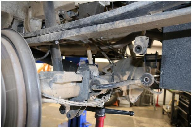
11) Use a pair of quick clamps or C-clamps to secure the main and lower spring together. See image below for reference.
