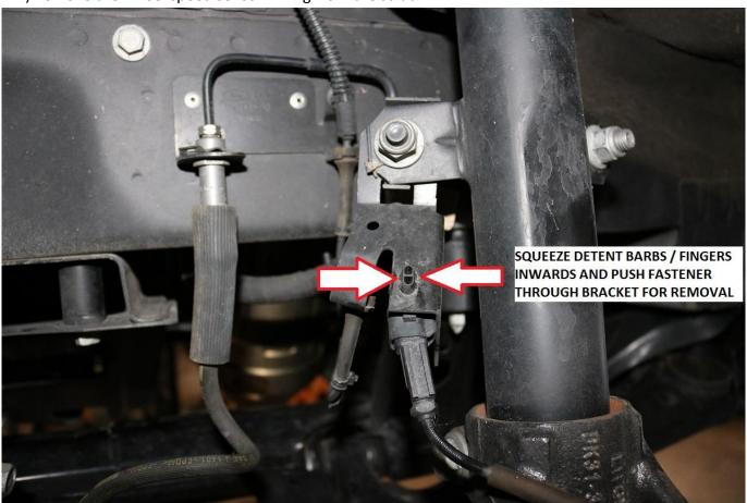
13) Completely remove the wheel speed sensor wiring from the strut. Separate the wheel speed sensor from the chassis harness.
