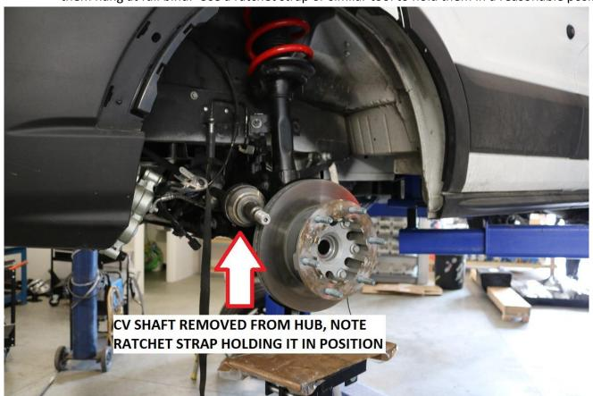
20) With the CV free from the hub, support the steering knuckle with a transmission or floor jack and remove the 18mm lower strut bolt.
