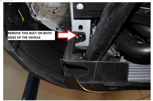
6) There are two bolts attaching these bars to the front suspension sub frame. Use a 13mm socket / wrench for removal.
