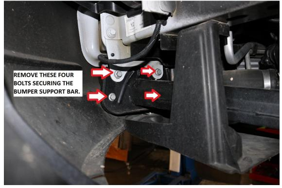
8) Remove the bumper support bars from the vehicle. This is a bit challenging but we have found the easiest way to do it is to move the front of the bars towards the outside of the vehicle and the back of the bars towards the inside of the vehicle. With some careful maneuvering, they can be removed without forcing them against the bumper or air damn.
