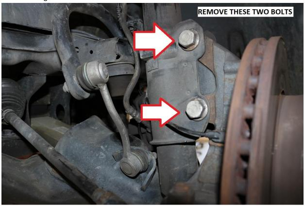
11) With the strut disconnected from the steering knuckle, allow the lower control arm to hang free again. Be careful to slowly lower the knuckle out of the strut. Be sure the wheel speed sensor wire and brake hose are not strained.
