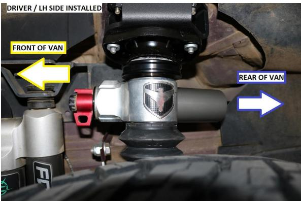
c. Install the upper strut bolt to hold the strut in place and prevent it from sitting on the CV boot on 4x4 / AWD models.
