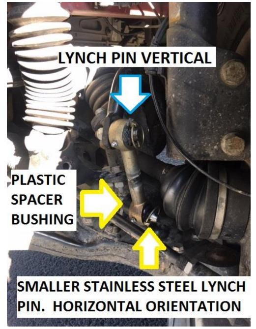
7) Re-check all bolt torques after 100 miles of driving. Grease the zerk fitting on the sway bar disconnect every 3-5k miles.
