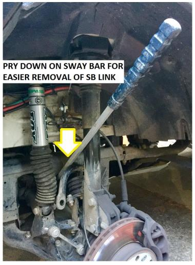
3) With the factory sway bar link removed, fit the smaller of the two sway bar disconnect studs into the swaybar itself. See image below for reference.
