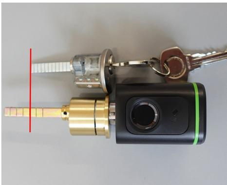
5. Align the keyed cylinder with the lock handle and mark the length of the tail.
