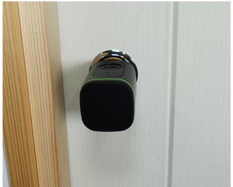
12. Installation complete. Rotate 180 degrees so that the sensor faces the floor.
