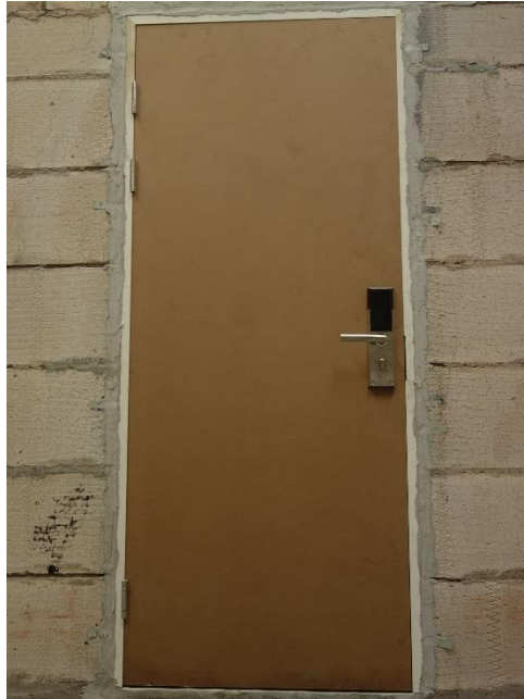
Fig. 1 Exposed Side Prior to the Fire Test
