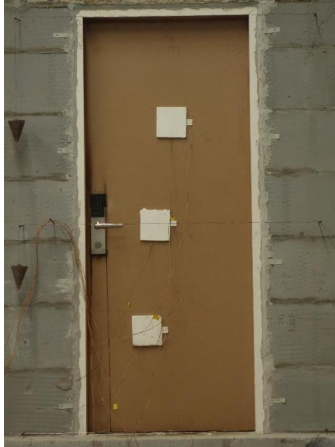
Fig. 3 Unexposed Side after 20 Minutes
