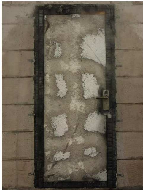
Fig. 8 Exposed Side after Hose Stream Test
