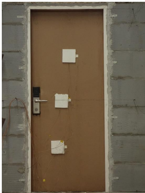
Fig. 4 Unexposed Side after 40 Minutes
