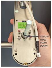
STEP 9 Take the outside lock body and insert the correct length spindle for your door and secure with the split pin. Where the spindle inserts, there is an arrow, this MUST point to the floor.
