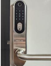
STEP 21 To wake the lock, sweep your hand across the face of the keypad. The numbers will illuminate
