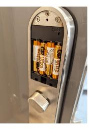
STEP 18 Insert 4 x AAA batteries (not incl) and fit the cover plate. Turn the thumbturn to check that it activates the deadbolt. Also make sure that the main handle retracts the latch.
