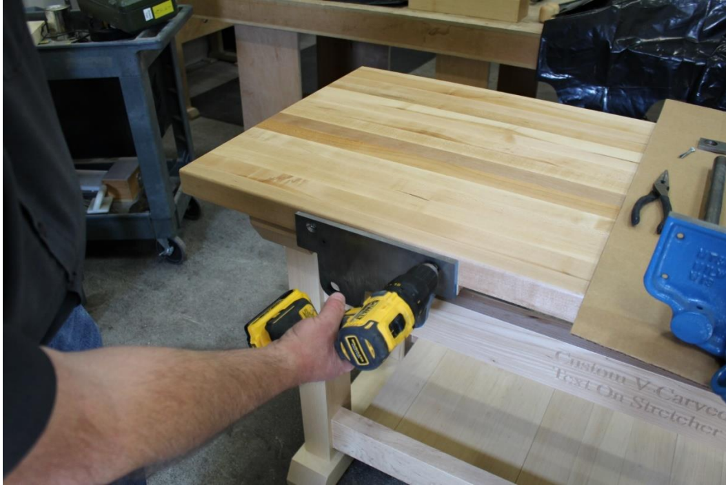
Step 7: Screw vise base unit into position on side edge of workbench top.
