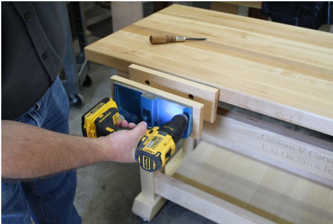
Step 14: Secure the vise jaw liners into position and attach accordingly with the proper screws. First attach the front jaw liner.
