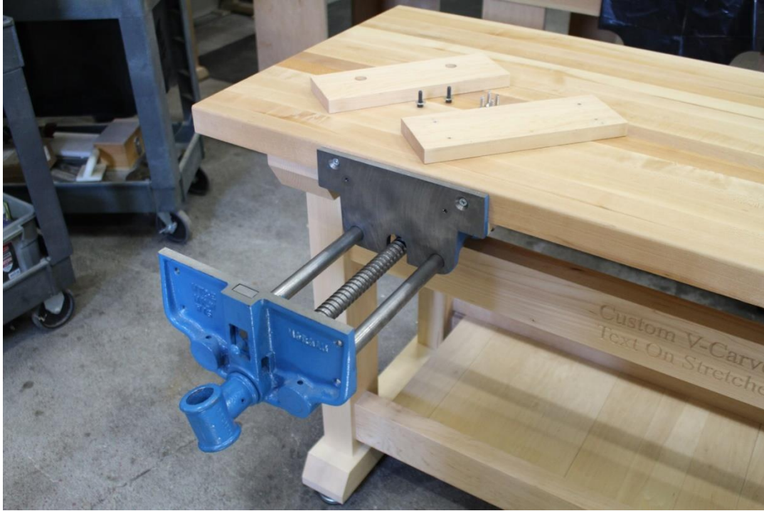
Step 13: Slide the vise unit out and then ensure that the vise nut engages properly into the vise.
