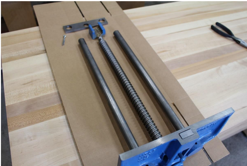
Step 8: Position quick release vise glide unit on bench top for easy install into vise base unit.
