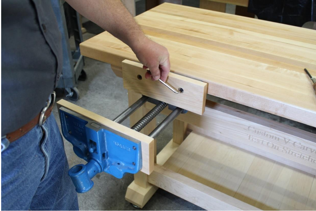
Step 15: Attach and secure the rear jaw liner.
