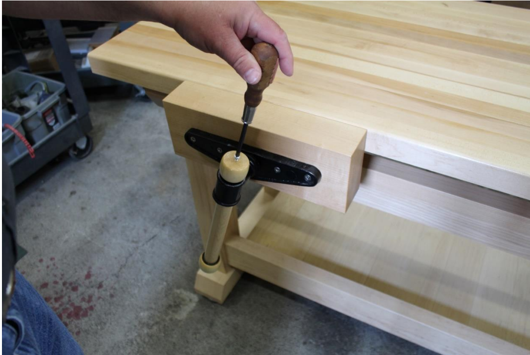
Step 9: Insert vise handle and secure using end cap screws on both handle ends.
