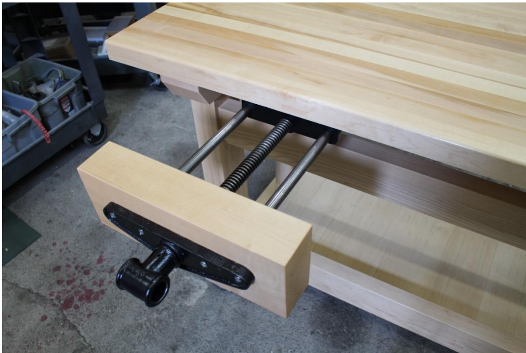
Step 8: Thread Vise/Jaw assembly into main vise casting.
