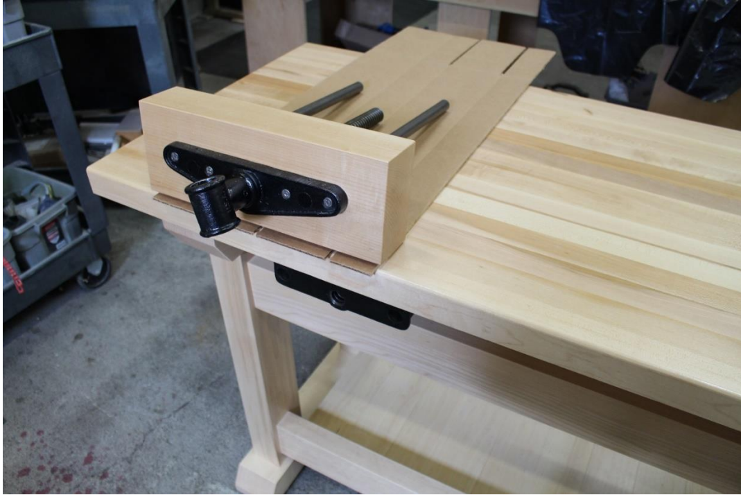
Step 7: Vise/Jaw assembly secure and ready for threading into main vise casting under bench top.
