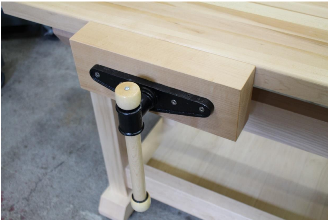
Step 10: Vise is completed and ready for clamping action. Job well done!
