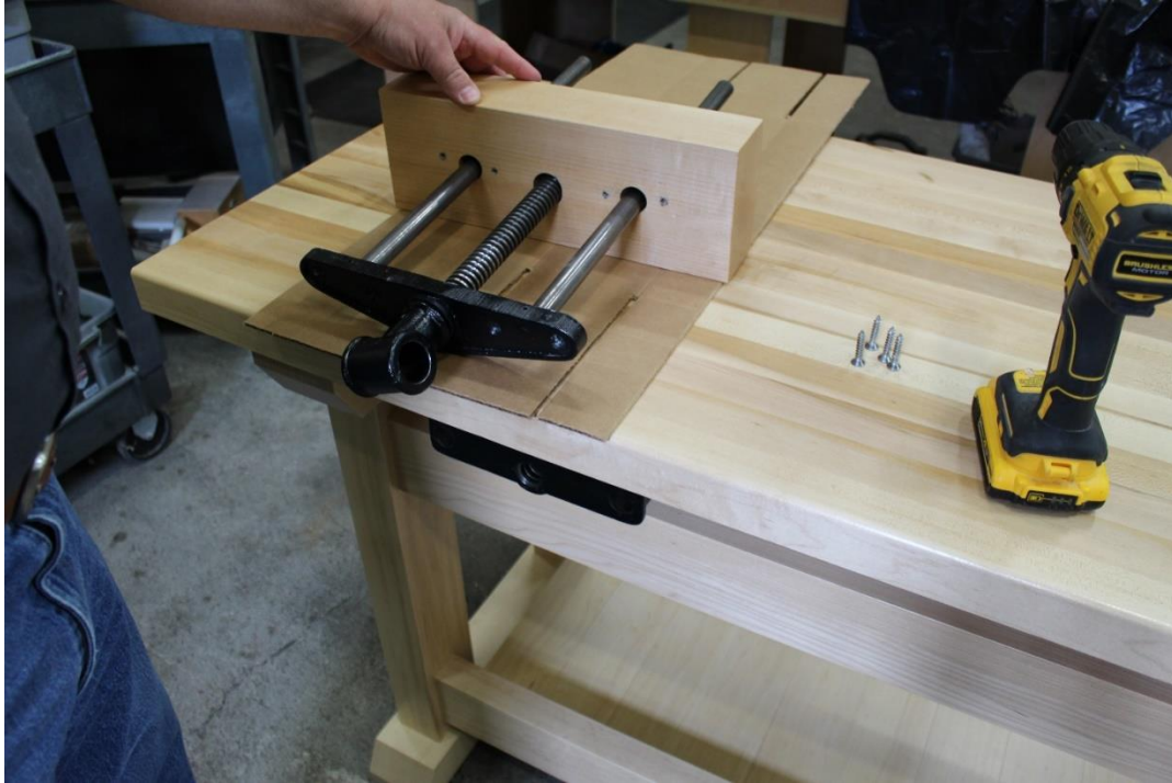
Step 5: Slide pre-drilled jaw liner onto vise screw/guide unit.
