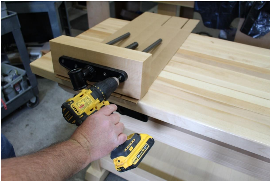
Step 6: Securely attach vise jaw liner onto vise screw/guide unit using proper sized screws.
