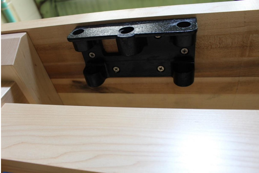
Step 3: Main vise casting securely fastened to underside of workbench top.
