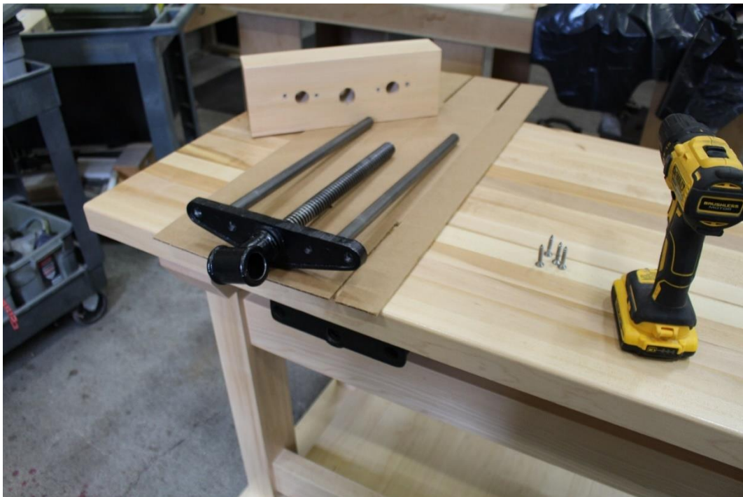
Step 4: Position vise guide/screw unit on bench top for easy install into vise jaw liner & vise casting.
