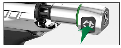
To remove the bolt, grab the bolt back cap with your right hand. Push the bolt release button, located on the left side of the bolt back cap, with your thumb. With the bolt release button depressed pull firmly back on the bolt.
