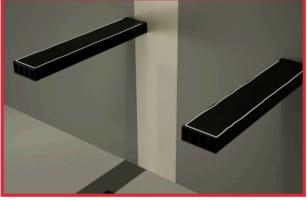
2. Install preferred backer board to manufacturer specifications. Then apply adhesive to both brackets.
