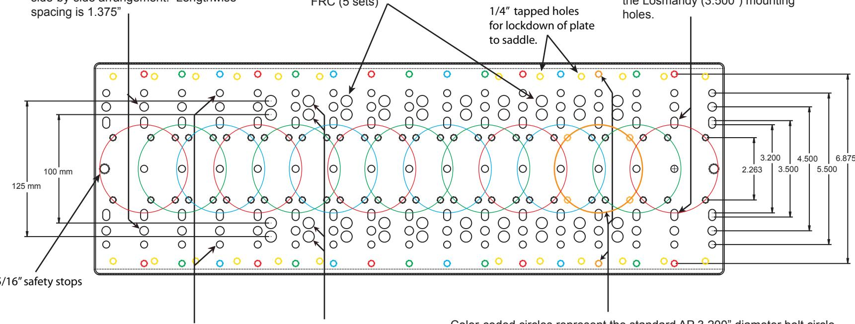
1/4" thru-holes with 5.500" crosswise spacing are available for custom applications. Lengthwise spacing is at 1.375" for the 5.5" sets.
