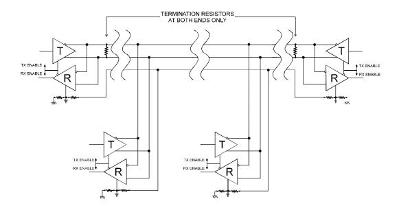
Figure A-1: Typical RS485 Two-Wire Multidrop Network
