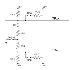
Figure 3-1: Simplified Schematic
