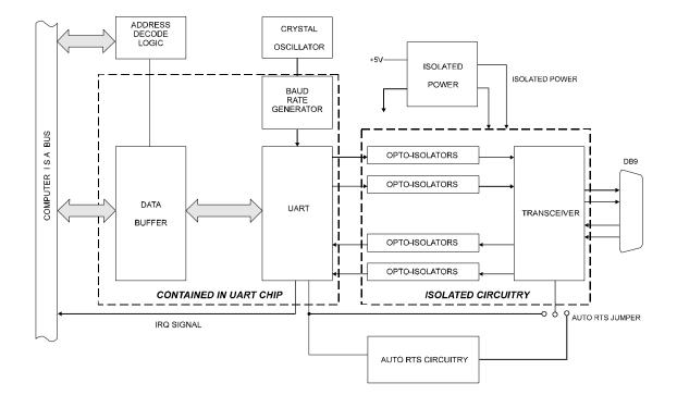
Figure 1-1: ICOM-2S Block Diagram (Only one serial channel shown)
