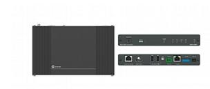
EXT3-C-XR-T is a high-performance, extended-reach HDBaseT 3.0 transmitter, with a USB-C input, for 4K60Hz (4:4:4) HDMI, USB, Ethernet, RS-232, and IR signals over twisted pair. EXT3-C-XR-T transmitter converts all input signals into the transmitted HDBaseT 3.0 signal. It extends video signals to up 100m (330ft) over CAT copper cables at up to 4K@60Hz (4:4:4) video resolution
