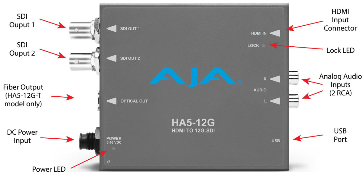
Figure 2. HA5-12G/HA5-12G-T Converter Connections
