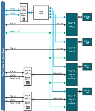
PCIe/104 is part of the PC/104 family of standards, and incorporates PCI Express, USB, SMBus and other data channels in the stack, not a single bus (ISA or PCI) as in previous standards. It is intended to be used in environments where a truly rugged computer system is required. PCIe/104 allows consumers to stack together boards from a variety of COTS manufacturers to produce a customized system ruggedized against the stresses of embedded environments.
