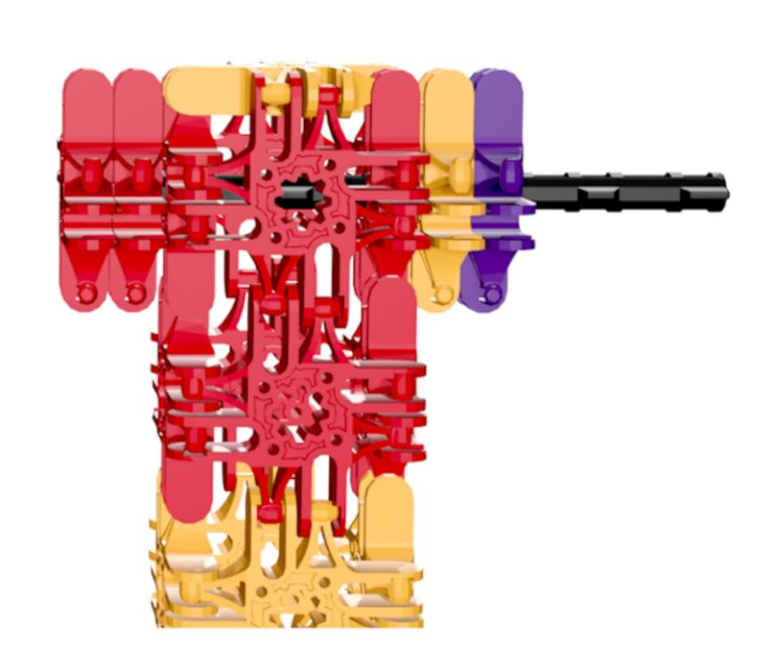
Side view for comparison, for next step push front axle out, leaving a gap between the two pillars
