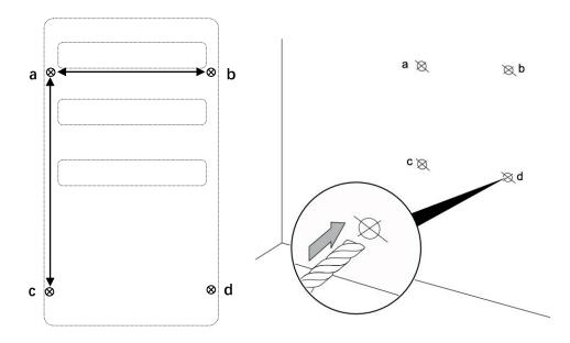
3. Drill the holes. Insert the Anchor (G) into 4 holes and use the screw (H) to tighten the Alloy ingots (C) onto the wall.
