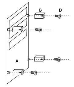
Affix the Towel Warmer to the Wall, Mark the bracket positions for the bore holes onto the wall.(Measure actual punching distanc of 4 brackets.
