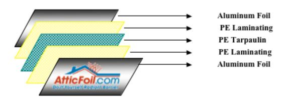
AtticFoil® solid, double-sided material structure: 3 layers of material + 2 layers of PE laminating
