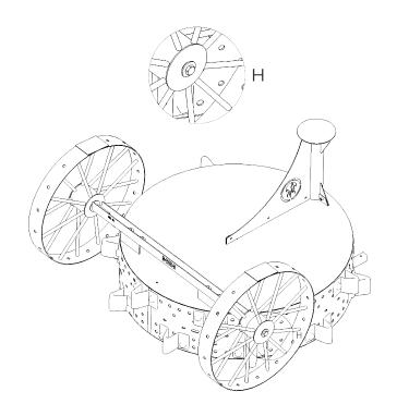
**Step 6:** Place the trim in position and fix the bolt M14 x 25mm with the M14 nut (included).
