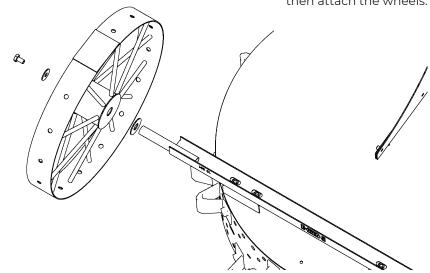
Step 5: Once the wheel is in position, place the M14 washer and fix the M14 x 25mm bolt (included).
