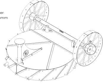
Step 6: Place the trim in position and fix the M14 x 25mm bolt with the nut M14 (included)
