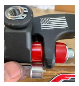
Flexx Handlebar Low Bar Elastomer Adjustment
