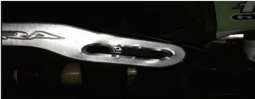
Now you can bolt the guard to the pivot pin. Depending on where you have your Flexx Handlebar positioned the guards may sit too high or low. You can easily adjust the angle or height of the guard by bending the portion of the guard that bolts to the handle either up to lower the guard or down to raise the guard. It is easiest to do by placing the inner portion of the guard in a vice and twisting the rear of the guard.
