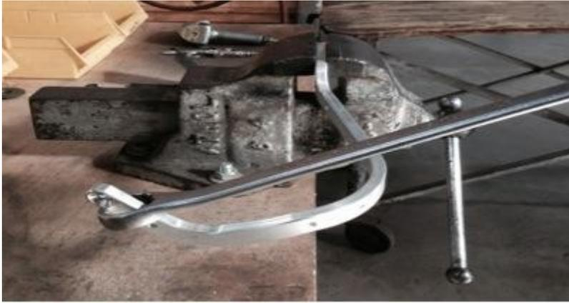
Twisting the guard towards the back of the bar will result in raising the guard.
