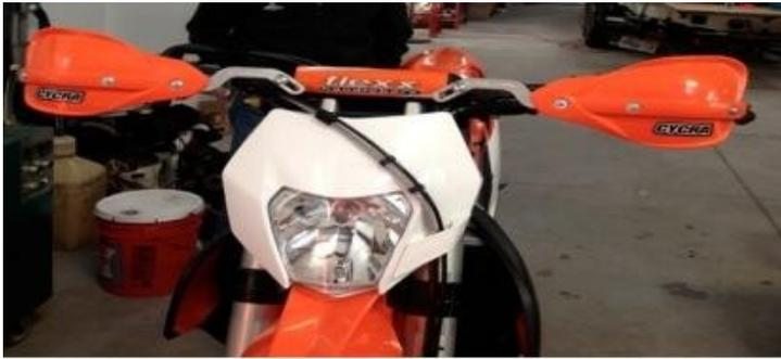
Mounting Cycra CRM guards is fairly simple if you have not trimmed your Flexx Handlebar narrower. We do suggest using our 10mm hand guard bolt and bushing kit ([CLICK HERE](#)) to mount the guard to the pivot pin. Our 10mm button head bolt minimizes the ability for your lines to snag on the bolt head. We also suggest using threaded anchors to secure the guards to the handles. Shown below is the 10mm button head bolt and bushing kit as well as our threaded inserts.
