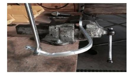
It may take a few tweaks to get the guard to sit at an acceptable height. Once you have it where you would like it tighten up the bolts and you are ready to ride. We suggest using a drop of blue loctite on the 10mm bolt.
