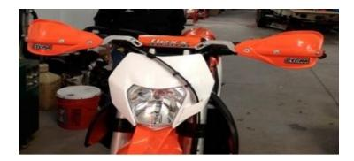
Mounting Cycra CRM guards is fairly y simple if you have not trimmed your Flexx Handlebar narrower. We do suggest using our 10mm hand guard bolt and bushing kit (CLICK HERE) to mount the guard to the pivot pin. Our 10mm button head bolt minimizes the ability for your lines to snag on the bolt head. We also suggest using threaded anchors to secure the guards to the handles. Shown below is the 10mm button head bolt and bushing kit as well as our threaded inserts.
