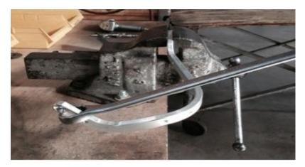
Twisting the guard towards the back of the bar will result in raising the guard.
