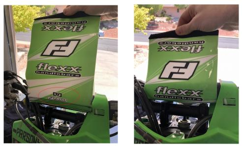
3. At this point, wrap the pad cover around the foam and start to secure the Velcro.
