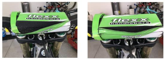
5. Once you have the Velcro strip securely fastened, now roll the bar pad cover so the logos are properly oriented on your bar pad. The Flexx Handlebar logos should be on the front and back of your bar pad, while the FF logo (FasstCompany/FlexxHandlebars) will be on top. If done properly, your bar pad should look similar to the photo below.
