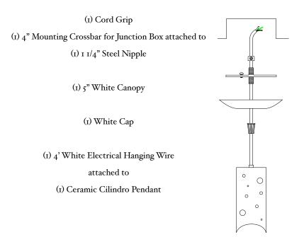
Slide the White Cap, White Canopy, Mounting Crossbar and Steel Nipple, and Cord Grip over the White Electrical Hanging Wire.
