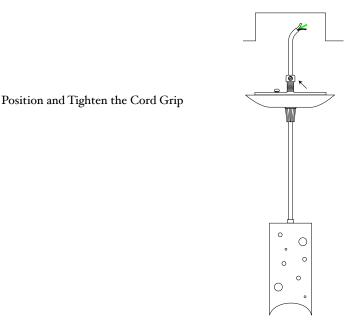
Attach the Mounting Crossbar to your Junction Box using the screws in your Junction Box. Cut any excess Electrical Wire length, strip the wire ends and attach to your power source.
