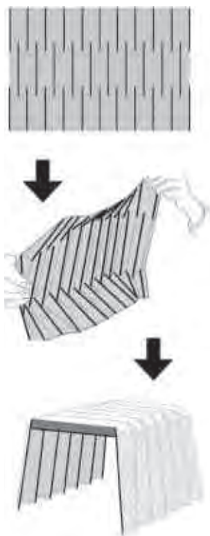
[Abb. 3] Illustration zum Tragsystem des Pavillons. 2012.
