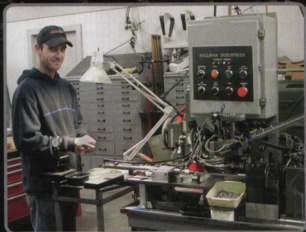
Above: Jeremy McCoy inspects Innerloc broadhead tips as they come off one of Sullivan's custom-built, tip-producing machines.
