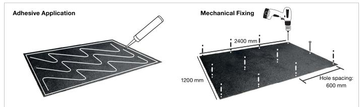
When fixing COBAGRiP® Sheet, drill holes in all 4 corners with additional holes for fixings approximately every 600 mm. Holes need to be located 70 mm away from the front edge and 60 mm from the back edge.
