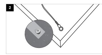
The male stud is incorporated into the mat and attaches the Floor Mat with the Floor Mat Grounding Wire.
