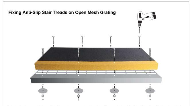
Install using the same fixing points above, then use universal saddle clip assemblies with slotted truss head bolt, nut and lock washer (all stainless steel).
