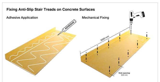
The fixing points for COBAGRiP® Stair Treads need to be in all 4 corners, with additional holes for fixings approximately every 600mm. Holes will need to be drilled 70mm in from the front edge and 60mm in from the back edge.
