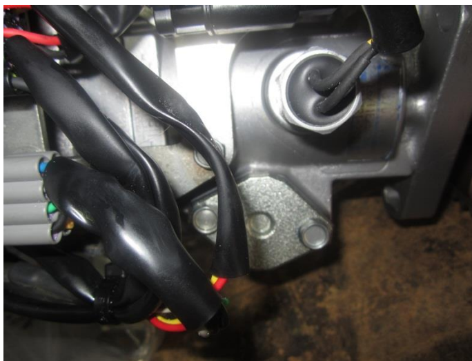
Pictured above: Pump with dimple advance plate
