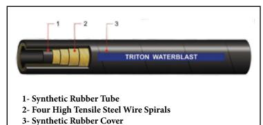
**Tube:** Oil resistant, synthetic rubber **Reinforcement:** Multiple Spiral Technology **Cover:** Oil and weather resistant synthetic rubber **Temperature:** -40° F / +213° F, Intermittent use up to 250° F
