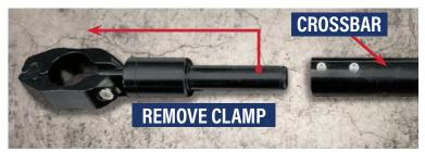
**CAUTION:** The Set Screws are Tiny! Be careful where you insert the set screws into the handlebar crossbar. Do it over a table or an area where it will be easier to notice the screws if they fall onto the ground.
