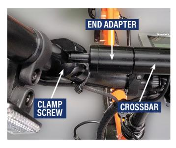
Place the end adapter between clamps A and B. Insert the clamp screw and slightly tighten clockwise with the 4mm Allen key.
