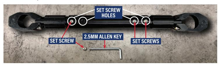
CAUTION: The Set Screws are Tiny! Be careful where you insert the set screws into the handlebar crossbar. Do it over a table or an area where it will be easier to notice the screws if they fall onto the ground.
