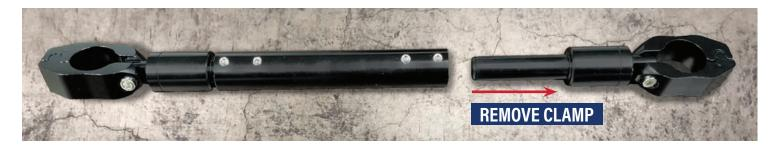
Using the 4mm Allen key, turn the clamp screw counterclockwise to remove the screw from clamps A and B.
