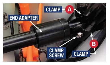
Place the end adapter between clamps A and B. Insert the clamp screw and slightly tighten clockwise with the 4mm Allen key.
