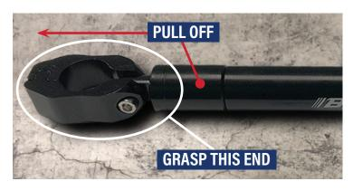
Grasp the other end of the handlebar clamp and pull the adapter clamp out from the crossbar. You will need the crossbar in the next step.
