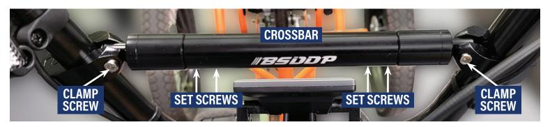
At this point, the crossbar should be on the handlebars but most likely uneven. The last two set screws should be loose. Loosen all the other set screws, just enough, so that you can make any adjustments.
