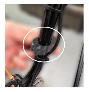
Stand in front of your Liberty Trike. Place clamps A and B on the vertical section of your handlebar (circled in white). Make sure to place the handlebar clamp under any zipped cables tied to your handlebars.
