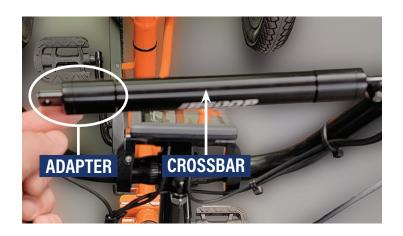
Insert the end adapter into the crossbar and slightly tighten the two set screws.
