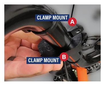
Stand in front of your Liberty Trike. On the opposite side of the handlebar, place clamps A and B on the vertical section of your handlebar.
